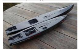
one metre long boat with a maximum width of only one hundred millimetres. I had a wooden planked hull made locally and it was fitted with a fixed DF65 fin and rudder. It did carry a heavier, 900 gram keel bulb and had a larger rig, whilst the standard DF65 A rig slotted in nicely as a B rig. It looked a bit weird but it would give us some idea if the idea of a long waterline,
